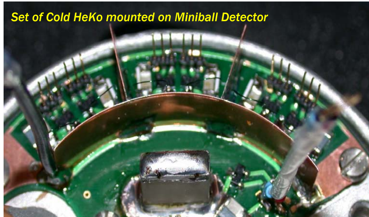
Technological steps in building - mounting a set of cold parts of CSPs on a 6_fold segmented encapsulated Miniball Detector
