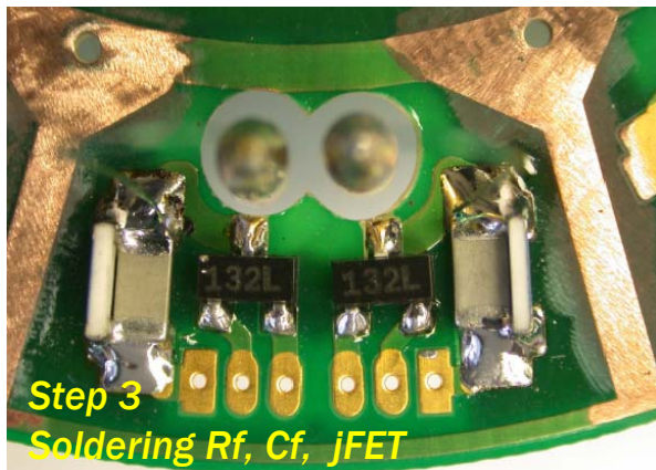
Technological steps in building - mounting a set of cold parts of CSPs on a 6_fold segmented encapsulated Miniball Detector
