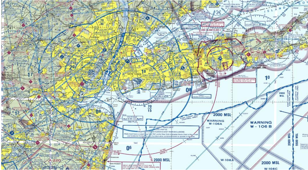
Fig. 2.4.1: New York City Terminal Control Area comprising JFK (Kennedy), EWR (Newark) and LGA (LaGuardia) airports from the NYC sectional aeronautical chart.
