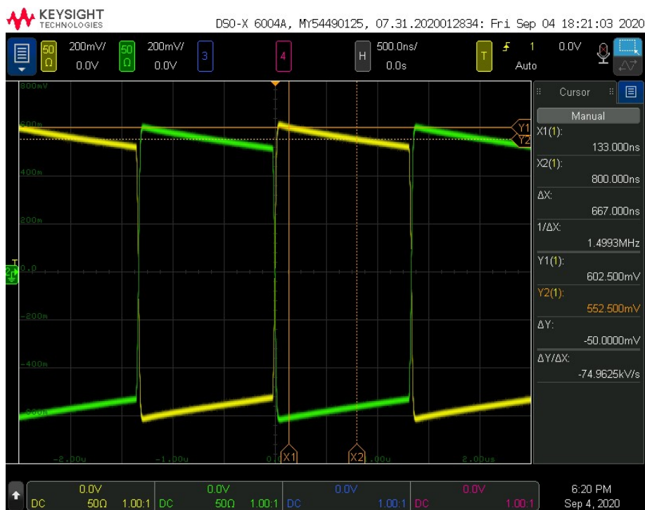
Figure 17: Voltage droop measurement on the oscilloscope with PHY Chip in testmode 2
